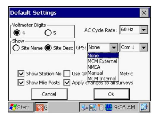
**Step 4:** Select the "NMEA" option and select "Com 1", which is the built-in serial port located under the flap on the bottom left hand side of the Gx data-logger.
