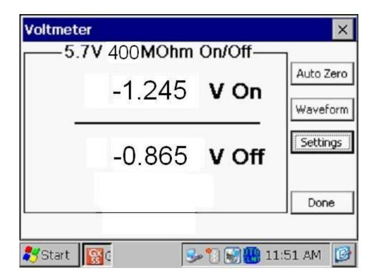
In the above case, the "stand-alone" voltmeter is reading the On and the Off pipe-to-soil voltages at a test station with the "Range" and "Input Impedance" values selected as 5.7V and 400MOhm, respectively.
