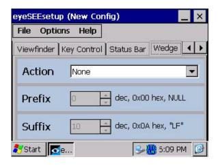
**Action** – Selects the wedge action to perform. Available selections are; *None*, *Send file name*, and *Send file path and name*. Selecting *None*, disables all wedge action. Selecting *Send file name*, causes the image file name to be sent to the active form. Selecting *Send file path and name*, causes the full file path to be sent to the active form.
