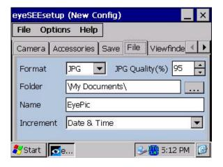
**Format** – Selects the image file format. The available selections are: BMP or JPG. BMP files contain uncompressed pixel data. The image data in a JPG file is compressed according to the JPEG standard. The file name is automatically given an extension based on the file format.
