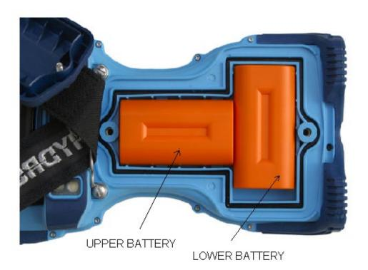
4. Remove the lower battery first, by sliding it to the left, at which point it should lift out easily. To remove the upper battery, slide it down
