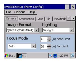
**Image Format** – The image format determines the size and resolution of the image. The available selections are: *QSXGA* (2048x1944), *SXGA* (1280x960), *VGA* (640x480), and *HF* (300x200) where the numbers in parentheses are the size of the image in pixels.
