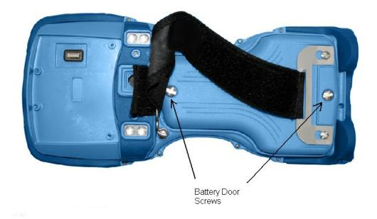
3. Unscrew both screws and remove the battery door. Both lithium-ion batteries will be revealed as shown below.
