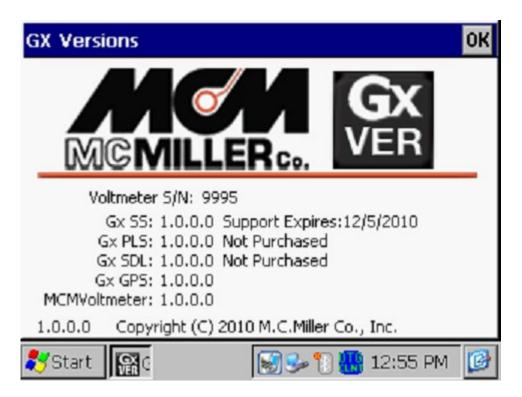
The above example screen indicates that the Gx\_SS (Test Site Survey) application has been purchased and that the expiration date for its support is 12/5/2010.
