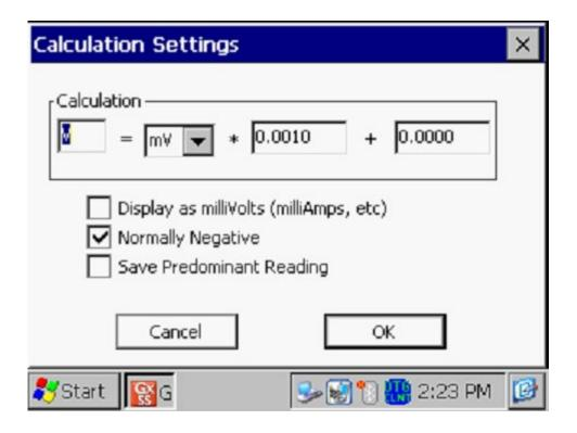
You could, for example, change the type of reference electrode you were using, in which case you would enter an appropriate value for the "addend".
