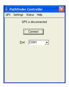
You should then select the appropriate COM port (COM 1 if using the serial cable).
