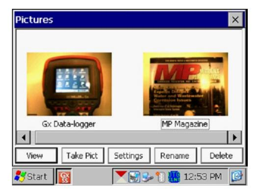
If you would like to adjust the camera settings from their default settings you can do so via the "**Settings**" button on the Pictures screen. For example, you can change the size and resolution of the image to be captured, the lighting conditions under which the image will be captured and the focusing method to be used, for example.
