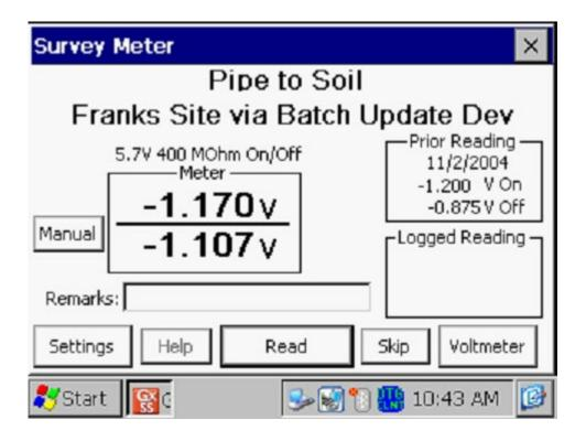
The voltmeter's "Range" and "Input Impedance" settings that were scripted on the ProActive side for this prompt are indicated below the test site name. As can be seen from the above screen, the data-logger is reading the ON and OFF pipe-to-soil voltages at the Valve test site. These voltages can be compared to the readings that were logged previously (on 11/2/04) at this site (see "**Prior Reading**" field). When the current readings are logged by
