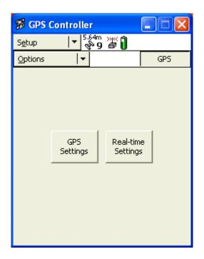
**Step 11:** Click on the "Options" drop-down on the above screen and select "Disconnect from GPS". Your NMEA settings will be transmitted to the GPS receiver upon disconnecting. The GPS receiver is now configured for use with the Gx data-logger
