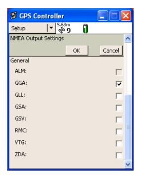
Next, make the selections indicated on the screen above (left-hand side screen). Next, use the scroll bar to scroll down to reveal the screen shown above (right-hand side screen) and select GGA only as the NMEA string type.
