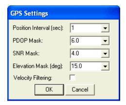
Based on the discussion in Step 7, we require position data to be output every second and so, your selection of "Position Interval" on the above window should be 1 second.
