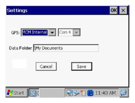
By tapping on the menu button in the GPS field, you can select the type of GPS receiver you are using. You can select either the "MCM Internal" receiver (if you plan to use the built-in GPS receiver on the Gx) or, an external "NMEA" compatible receiver (if you plan to use an externally-connected GPS receiver).
