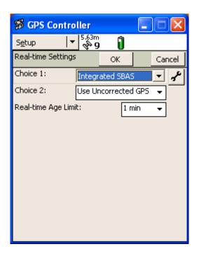
Next, under "Choice 1", select "Integrated SBAS" (which is WAAS differential correction) and click on the "wrench" button, which will pull up the screen shown below.
