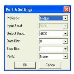
Select the output baud rate for the receiver and the other communications settings required to match the Gx's requirements.
